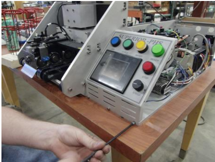
Figure 1: Remove control cabinet cover. Remove front panel.
