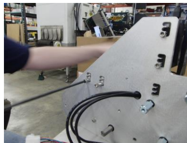
Figure 7: Remove top 2 screws on left panel to completely remove hold down assembly.
