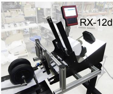
RX-12c/cs/d SPECS: Product sizes: 2"W x 3"L—12"W x 12"L. Product thickness: .004" - .375". Maximum belt speed: 400 ft./min. Maximum stack height: 16-in. Utilities requirements: 115vac—3A—60Hz (220vac—50Hz optional).
